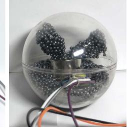
The programming is coded with Arduino setting the intensity of the attraction of the electromagnet according to the hardness of the shake on the sensor.
